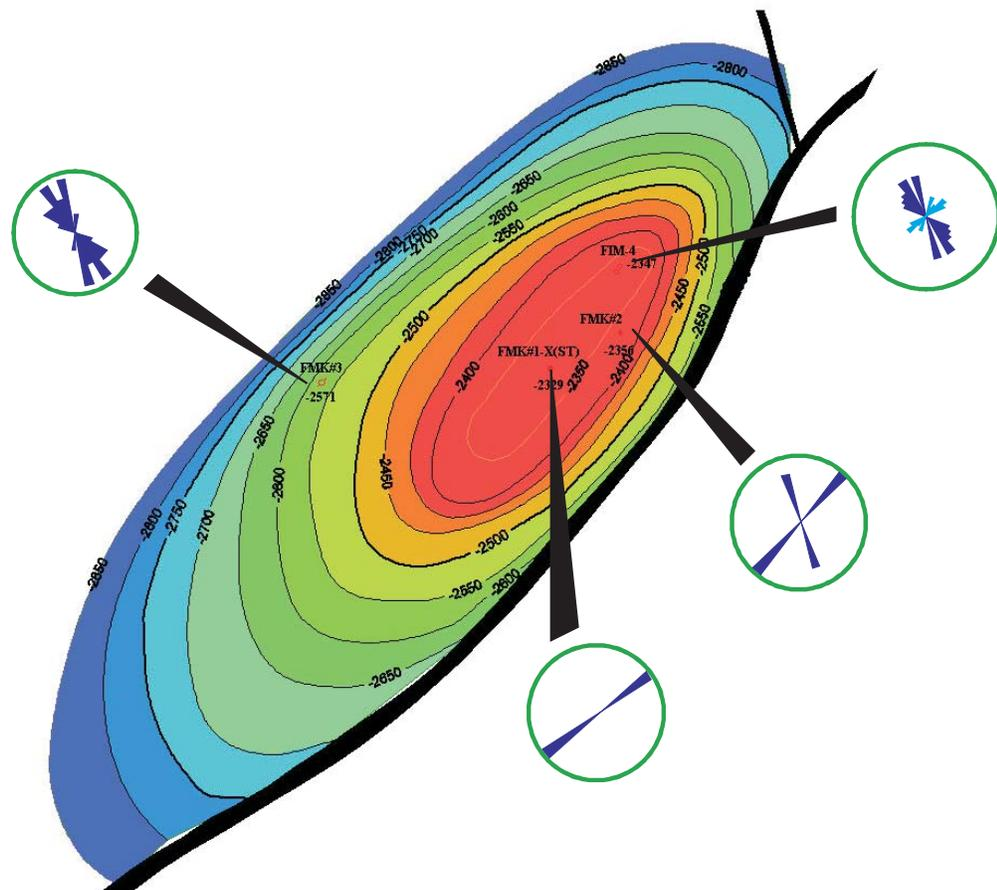
Figure 6- Fracture Orientation in four well.
