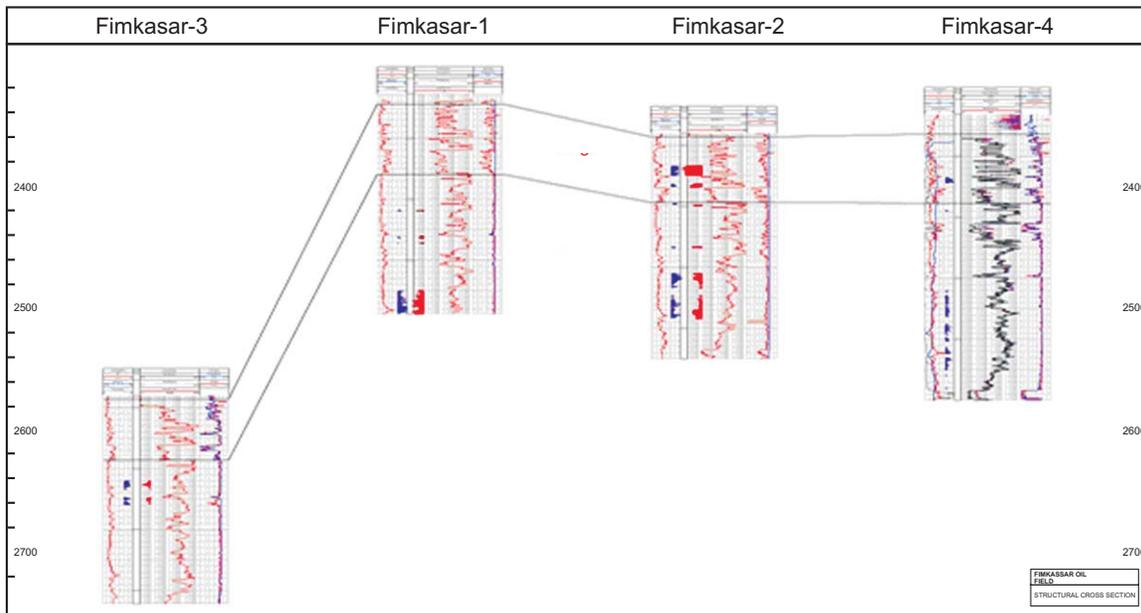
Figure 2- Structural correlation of the wells with fracture density.
