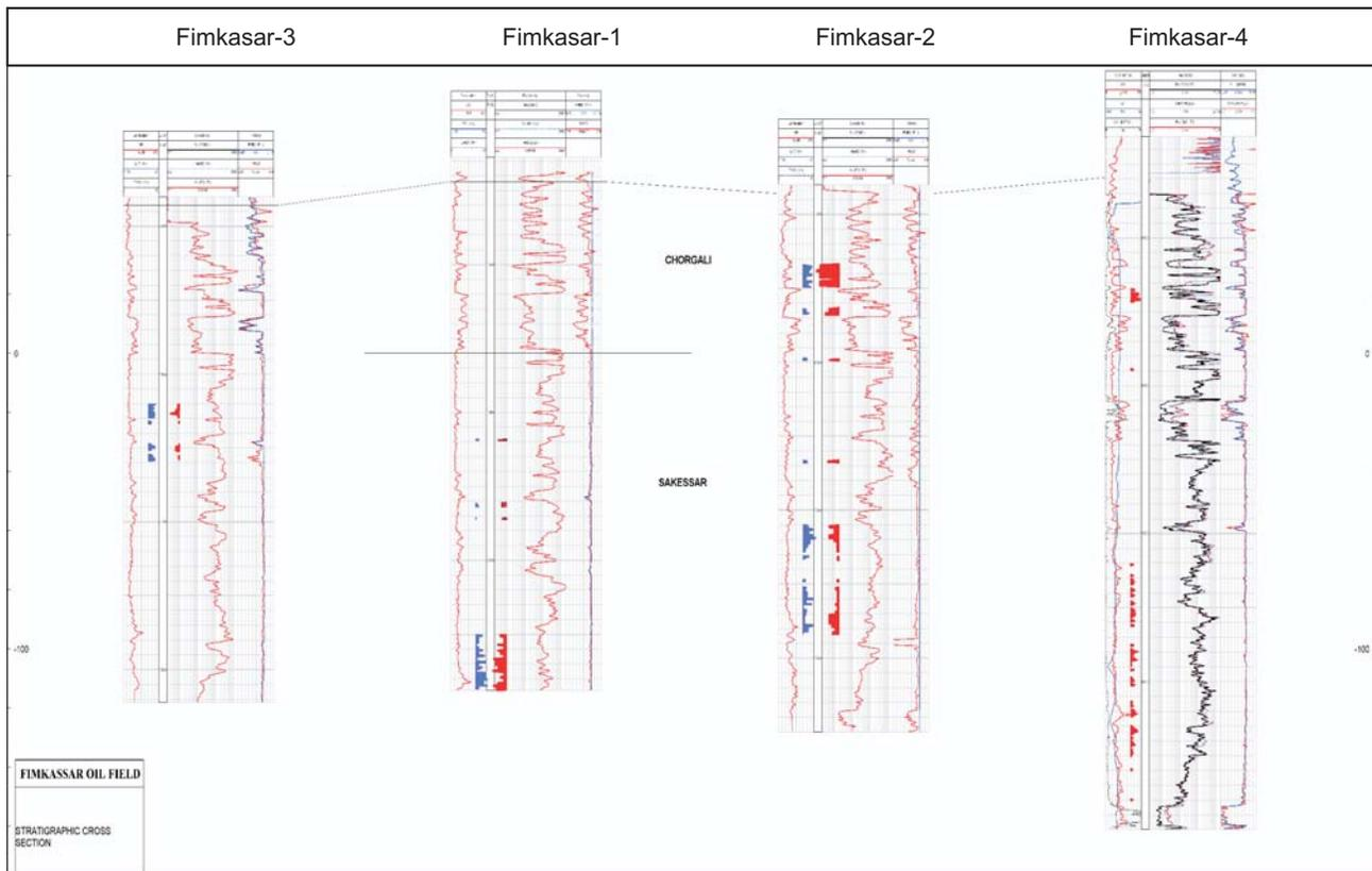
**Figure 9- Fracture density in four wells of the field.**
