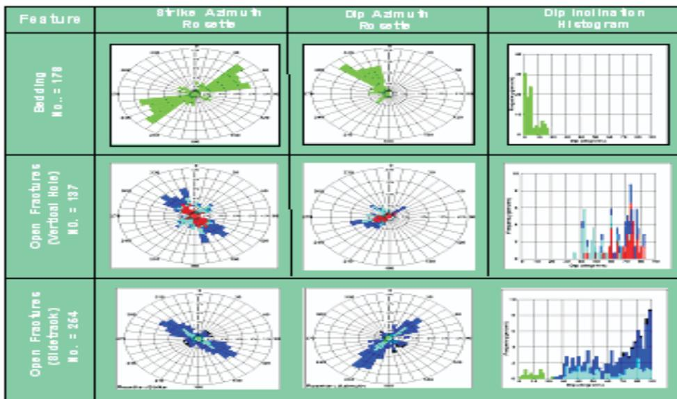
Figure 7- Rose diagram showing fracture orientation and other feature.
