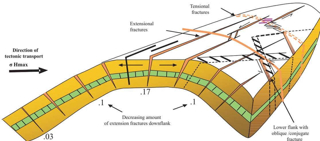
Figure 10- Fracture model of a folded structure (I. A.K. Jadoon et al 2005).
