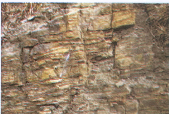
Plate 5A - Photograph displaying rippled/flaser-bedded lithofacies of Warchha Sandstone, Choa-Khewra Road Section (pen for scale).
