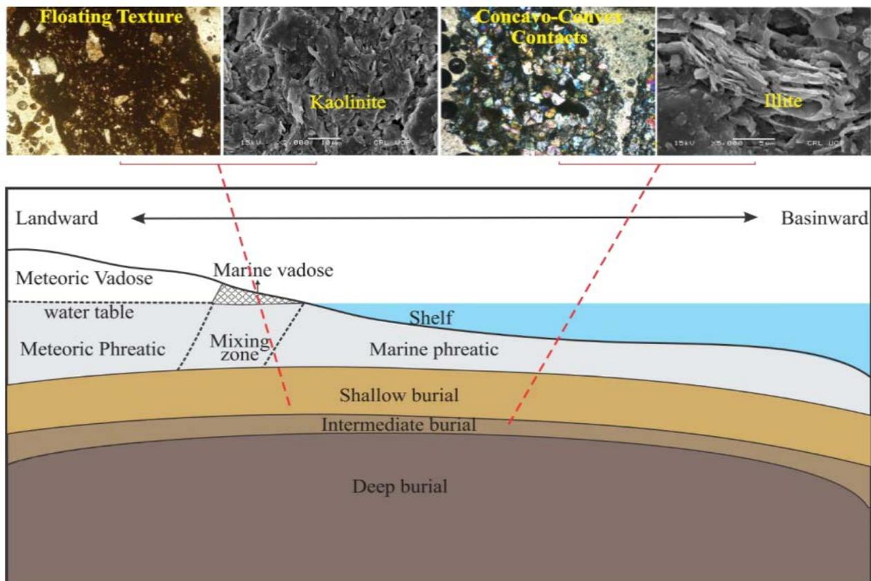
Figure 7 Diagenetic environment model for the Tobra Sandstone
